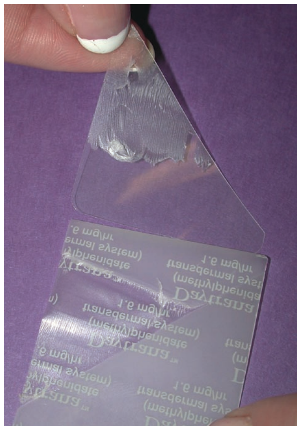
Figure 3. Half of the release liner manually removed from the Daytrana™ patch; adhesive remains on the release liner that was removed. (This lot was later recalled by Shire).
